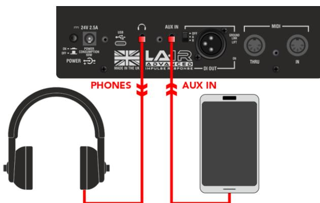
The SUPERGRACE includes a high-quality headphone output for silent practice. It is optimised for high impedance headphones such as common  $33\Omega$ , though any may be used.
