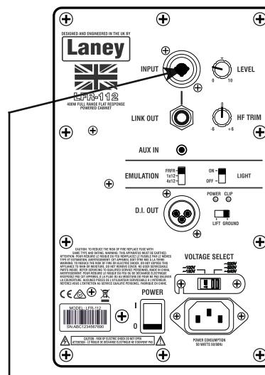
Main output from sound source. For mono use Left(mono). For a stereo rig use left(mono) & right to independant LFR-112 cabinets
