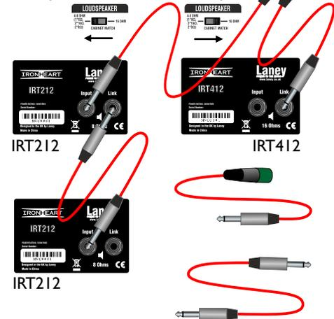
The IRT-SLS can be connected to your chosen cabinet via Speakon to jack, or jack to jack connectors in either a single or multiple cabinet configuration (as shown above).
