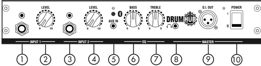
**Input 1 jack & mini jack inputs:** Sockets provided for connecting an external electronic drum/sound module. Use the regular input or the mini jack input depending on the output connections on your external electronic drum/sound module. Both accept a stereo or mono source.
