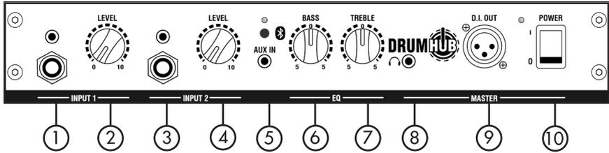
**Bass:** Adjusts the low-end response of the signal.
