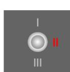
**II** - Similar character to the up position but driven even further to produce a more distorted tube sound. Even more asymmetrical clipping. Can be used to dial in a 'mild' to 'full' on bass distortion whilst remaining tight and clear. Experiment with the RANGE control to dial in your perfect sound.
