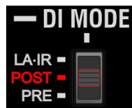
**POST** - The standard signal including FET/Tube channels, EQ and the FX loop. Not affected by master volume.
