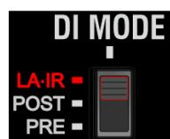
**LA-IR** - Same as post but will have the corresponding input IRs activated as well as any user EQ adjusted from the LA-IR app. Each input has its own preloaded IR, however these can be swapped out for your own via the LA-IR app.
