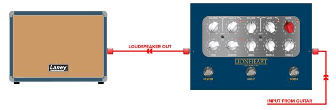
The BCC-LOUDPEDAL-LTQ can function just like your regular head, plugged directly into a passive speaker cabinet. Its loud.
