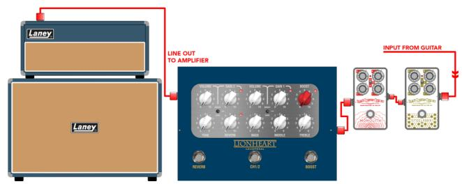
The BCC-LOUDPEDAL-LTQ can be connected in series with your regular pedal setup to act as a dual channel gain pedal with additional boost. Connect the FX send socket to your amp head.
