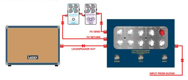
You can also connect your pedalboard to the BCCLOUDPEDAL-LTQ's FX loop and use the pedal in place of a regular amplifier. Output this to a minimum  $8\Omega$  passive speaker cabinet and you have your very own lightweight, portable amplifier.
