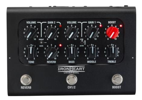
Thanks to its dual channel setup, the BCC-LOUDPEDAL-IMM allows you to easily switch between two tones set, via footswitch or MIDI. Each channel has their own Gain, Volume and Tone control with switchable BOOST and REVERB, again via footswitch or MIDI.
