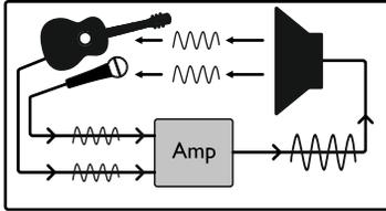
Audio feedback is caused when a loop occurs between a microphone or guitar pickup and the loudspeaker (see image to the right). Commonly caused by pointing a microphone at a speaker or simply by the two being too close. The result is an unpleasant screeching or whistling sound. The A-Solo is equipped to deal with this.
