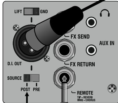
For additional level, or sound separation with left/right speaker system, the D.I from the first A-Solo can be connected Input of the second A-Solo. For best performance, use a balanced signal audio cable.
