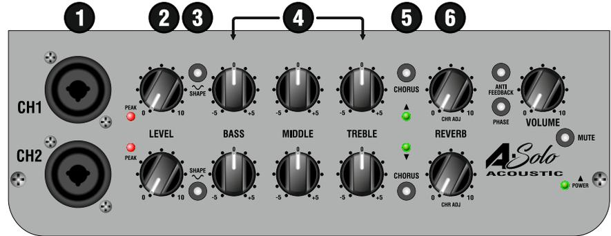
**2. LEVEL/PEAK:** Use together to find the optimum level for your signal. Adjust the Level so the Peak only lights during the very highest peaks of the connected signal.
