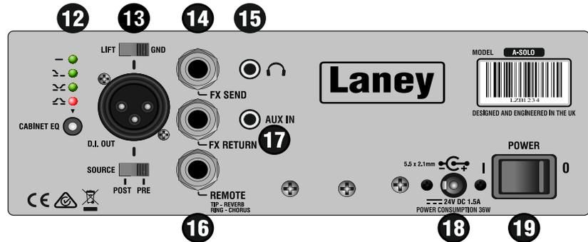
**13. D.I. OUT:** This socket provides a balanced output for direct injection of the amplifier signal into a mixing desk mic input. Using the Source switch, choose if the signal is Pre or Post EQ, FX and Mute. Refer to the block diagram on page 12. Finally, a ground lift switch is also provided to reduce the possibility of earth loop induced hum (when connecting to other equipment).
